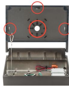
Easy installation options with integral wiring compartment. Mount directly over standard recessed or surface-mount junction boxes or use one of three 1/2" threaded conduit hubs for surface conduit mounting.
