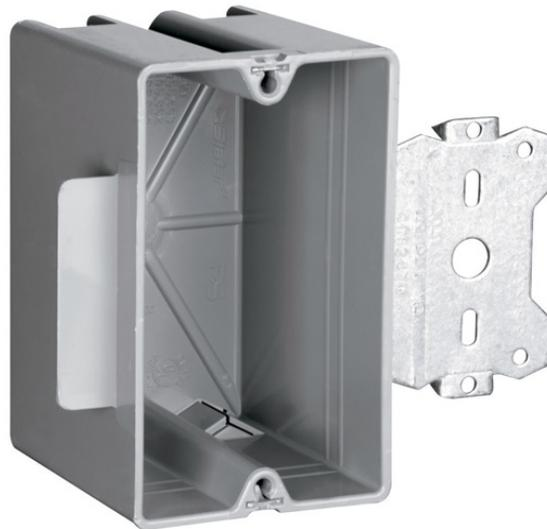
Single gang, wood and steel stud bracket box with 3/8" offset for wood and steel stud mounting. It has two Quick/Click Entries for each end, for use with 3/8" and 5/8" wallboard. It is available in single, two, three, four gang and 4 inch square boxes. It is molded of high-impact thermoplastic and can be used for steel, aluminum, or wooden studs. 100 pack.
