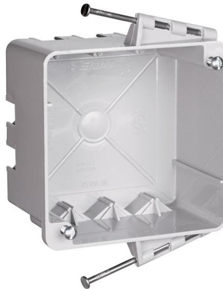
4" Square Box with Threaded Mounting Holes, Captive Mounting Nail each end. Three Auto/Clamps each end, Two on side adjacent to nails. Two #8 mounting screws factory installed.
