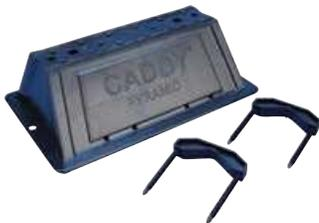
Provides a fixed height support 4" (102 mm) off the roof surface for outside pipe diameters between 0.50" – 2.38" (12.7 – 60.3 mm). Kits come in 5.5", 10" or 16" (140 mm, 254 mm, or 406 mm) lengths.
