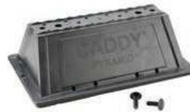
Provides a fixed height support 4" (102 mm) off the roof surface for cable tray. Kits come in 5.5", 10" or 16" (140 mm, 254 mm, or 406 mm) lengths with securing pins included.
