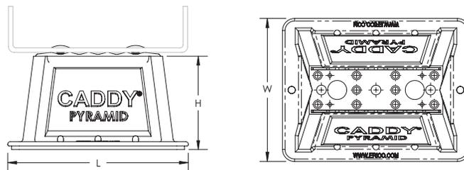
**NVENT CADDY PYRAMID TOOL-FREE PIPE CLAMP**
