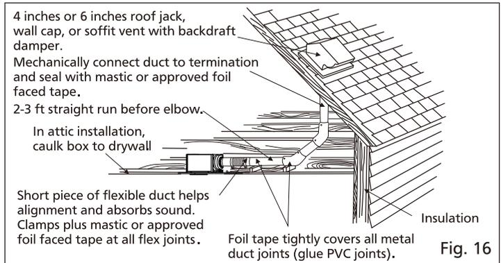
The ducting from this fan to the outside of the building has a strong effect on the air flow, noise and energy use of the fan. Use the shortest, straightest duct routing possible for best performance, and avoid installing the fan with smaller ducts than recommended. Insulation around the ducts can reduce energy loss and inhibit mold growth. Fans installed with existing ducts may not achieve their rated air flow.
