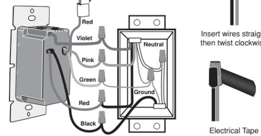
Connect wires per **WIRING DIAGRAM 1** (shown on page 2) as follows:
