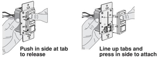
**Note:** Move slider on dimmer and slider on change kit to bottom of the slide bar prior to engaging.
