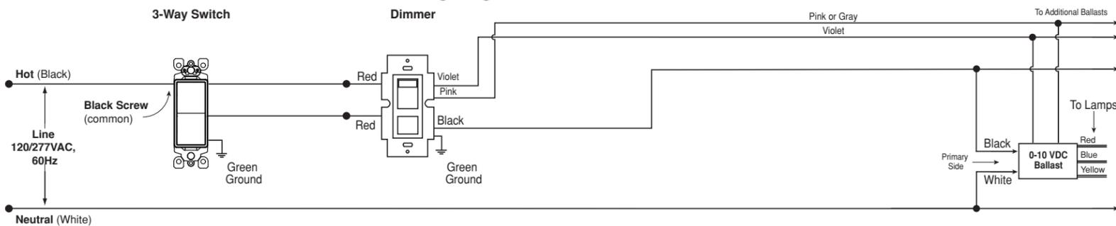
**Wiring Diagram 4: Two Location Control with OPP20 Power Pack**
