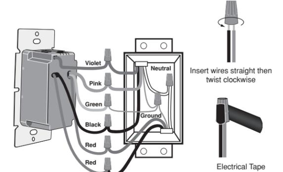
Connect wires per **WIRING DIAGRAM 3** (shown on page 2) as follows:
