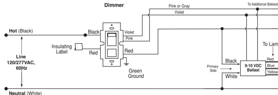
**Wiring Diagram 2 : Single Location Control with OPP20 Power Pack**
