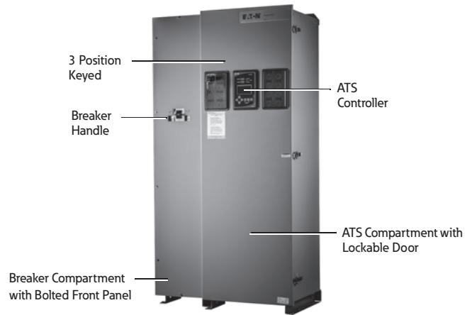
Typical Service Entrance ATS Construction for 600–1000 A NEMA 1
