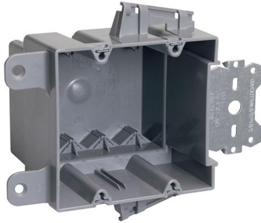
Double Gang, Wood and Steel Stud Bracket Box with Quick/Click, 3/8" offset for wood and steel stud mounting. Four Auto/Clamps on each end. For use with 3/8" to 5/8" wallboard. 50 pack.
