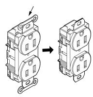
Note: If you do not see the perforation it might be necessary to snip the pieces off with a cutting tool. Avoid removing too much strap to maintain the integrity of the device mounting holes.
