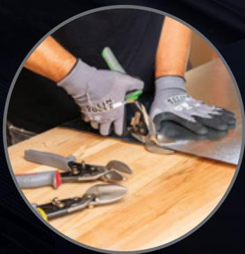
**CUTS UP TO 18-GAUGE COLD-ROLLED AND 22-GAUGE STAINLESS STEEL SHEET METAL**
