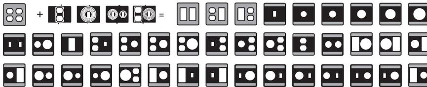
Multiple combinations of duplex, GFCI, switch and rounds: 1-3/8", 1-5/8", 1-3/4", 2-1/4", 2-5/8"
