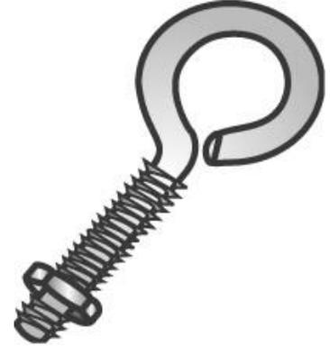
*An externally threaded fastener with a unified thread pitch and a blunt point. At the end opposite the gimlet point the unthreaded section of the shank is turned into itself in a circular shape.*
