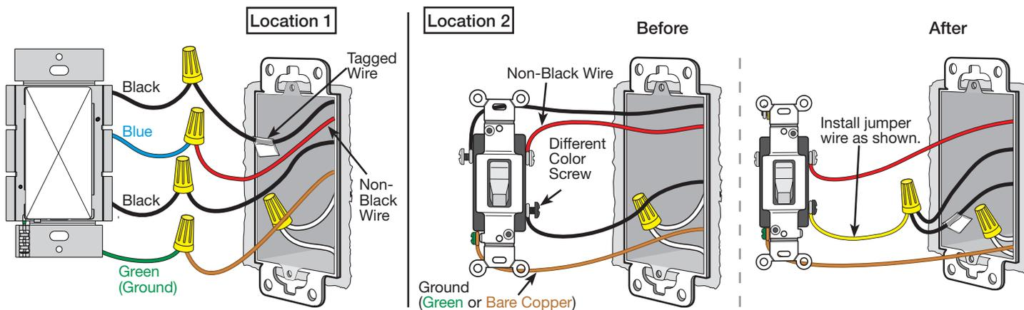
Note: If using a sensor switch, both ground wires must be connected for the sensor to operate.
